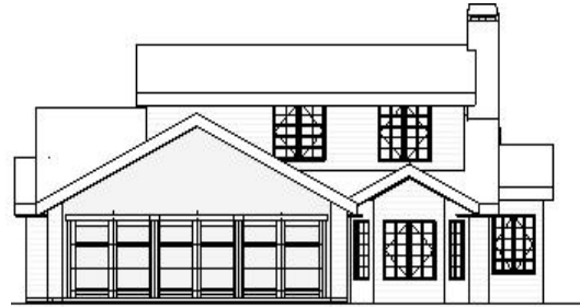
Figure 15 – Garage exceeds half the width of the front elevation.
